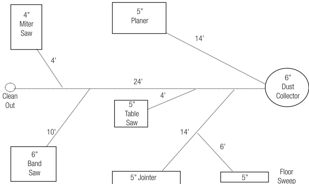
Illustrates a simple bird's-eye view of a 30' x 24' shop with the mainline duct running down the center of the shop.
