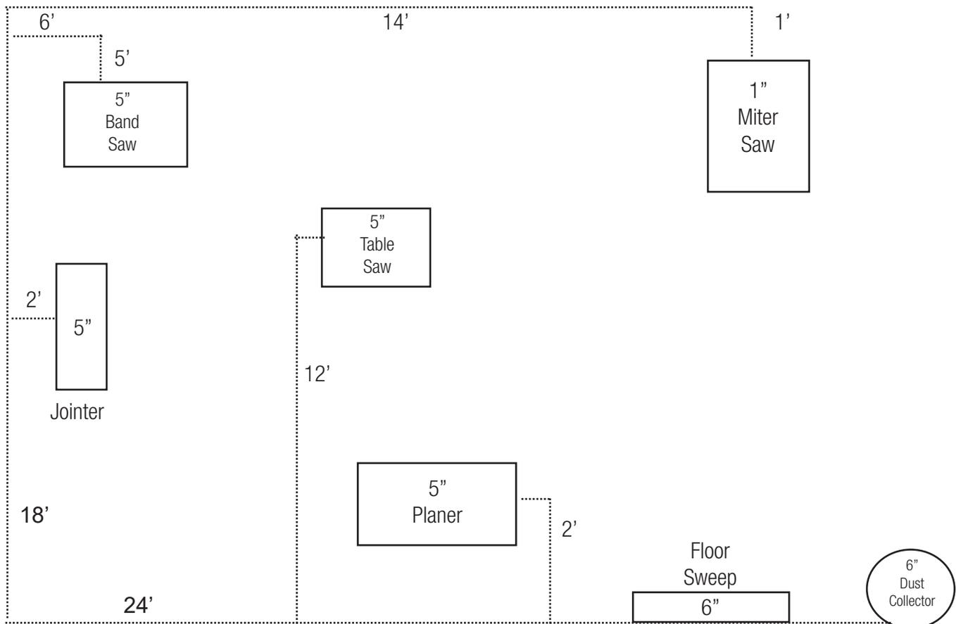
Illustrates a simple bird's-eye view of a 30' x 24' shop with the mainline duct running around the perimeter of the shop.
