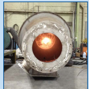
Heat curing of refractory at shop before shipment
