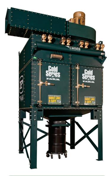
Farr Gold Series collectors feature a modular design for optimum field flexibility. Each module accommodates airflows up to 4,000 cfm using four cartridges mounted in a symmetrical frame. Additional modules may be added to meet total airflow requirements of 100,000 cfm and beyond.
