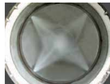
Liquid atomization in the high velocity zone maximizes particle impaction and capture of gas stream pollutants.
